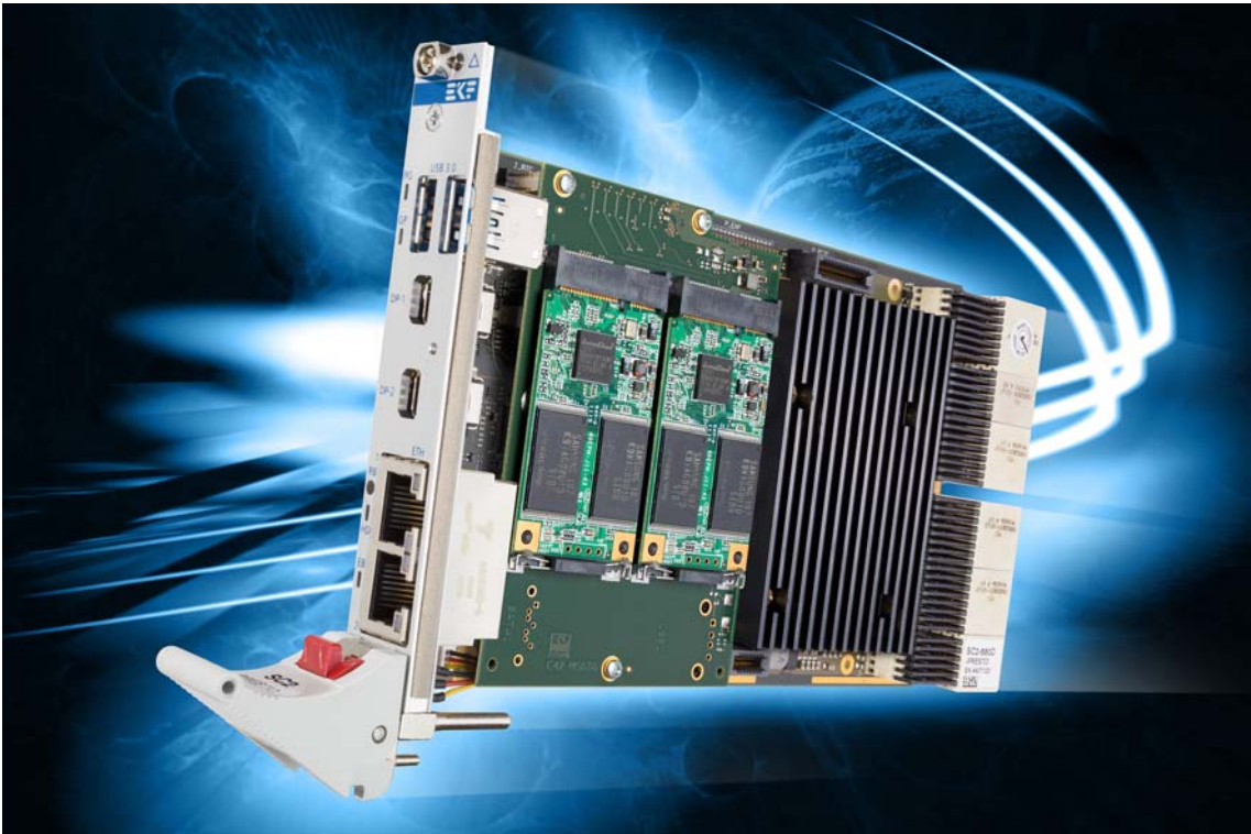
SC2-PRESTO w. C47-MSATA Mezzanine Module 4HP Assembly
