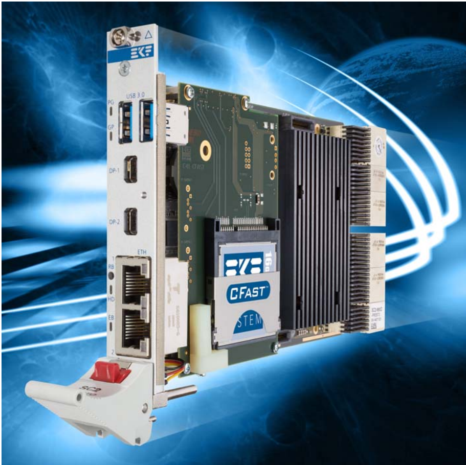
SC2-PRESTO w. C41-CFAST Mezzanine Module 4HP Assembly
