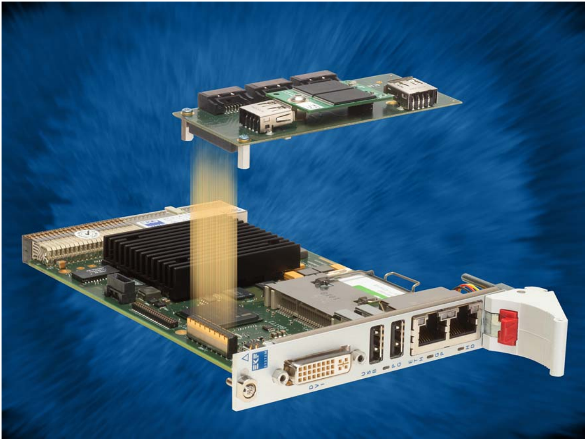
C43-SATA • Internal Connectors Mezzanine Module
