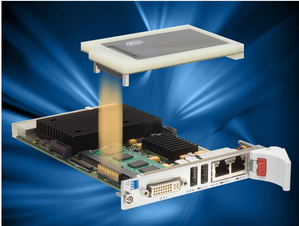
Expansion Connector J-HSE and Low Profile Module
