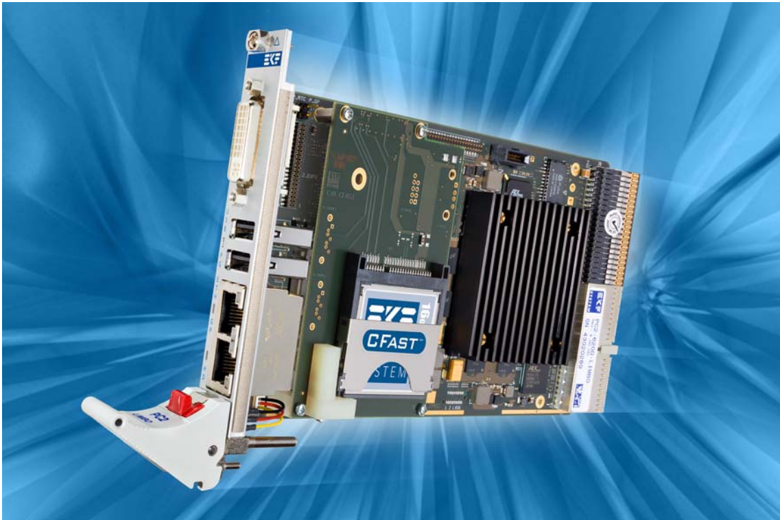
PC2-LIMBO w. C41-CFAST Low Profile Mezzanine Storage Module
